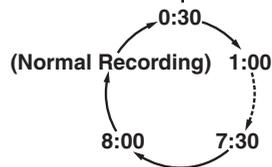
When the unit reaches the specified time, it will be turned off automatically.
