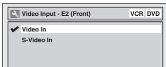
5. Using [▲ / ▼], select the input jack type to connect. Press [OK].
